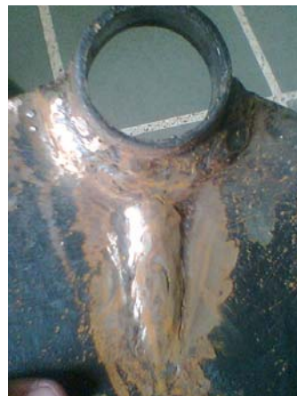
Fig. 28 (a) Eye hole for handle difference between existing and developed Courtesy Khidiya & Bhardwaj, Udaipur
