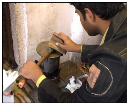
Figure 1. Heating & rolling lacquer lump in bangle manufacturing
