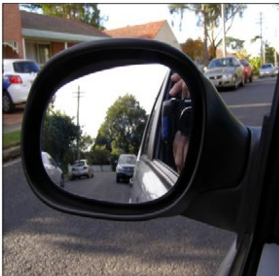
Figure 5: Example of the false visual information from convex side mirrors
